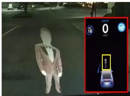
Figure 1: In practice, despite the fact that the Tesla Model X (HW 2.5) is equipped with radar and ultrasonic sensors, it recognizes a depthless person (phantom) projected on the road in front of it as a real obstacle due to its safety policy.
