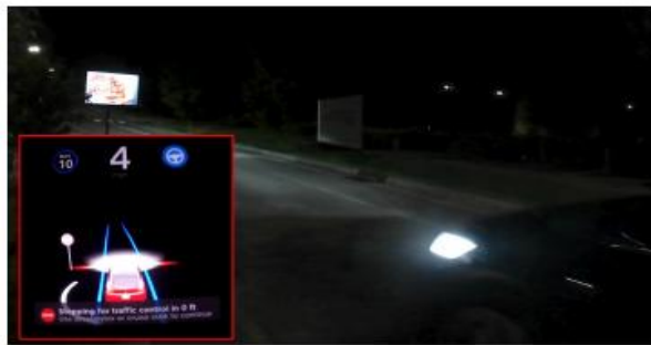
Figure 6: Tesla's autopilot triggers the car to stop suddenly after a phantom stop sign was detected in the upper left corner of the digital billboard.
