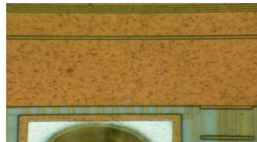
Top metal layer on microchip PIC16F877A microcontroller
