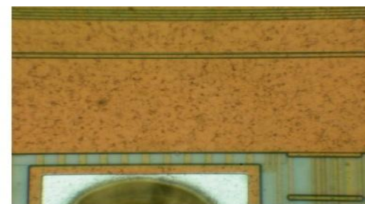
Top metal layer on microchip PIC16F877A microcontroller
