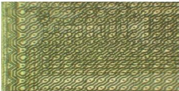
Top metal sensor on ST16 smartcard
