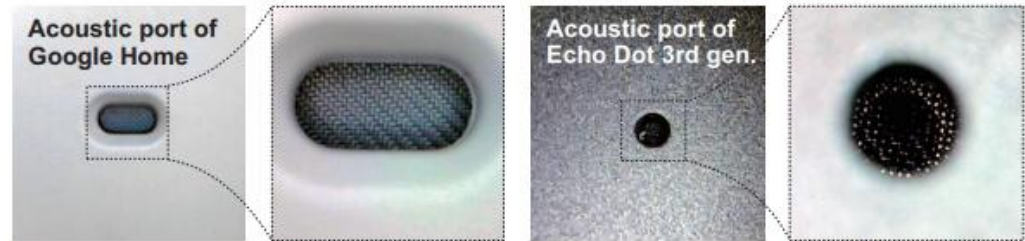
Fig. 3. Acoustic port of (Left) Google Home and (Right) Echo Dot 3rd generation. The ports are located on the top of the devices, and there are meshes inside the port.
